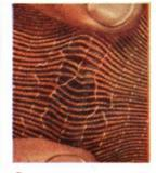
3 Most tire cords are bunched and gapped by slender cross threads. Weak spots, "slacker cords", overworked cords result. BFG cords, instead, are sealed in live rubber, with uniform spacing and tension.
